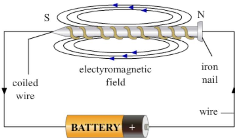
An electromagnetic filed is formed when a current passes through the wire.
